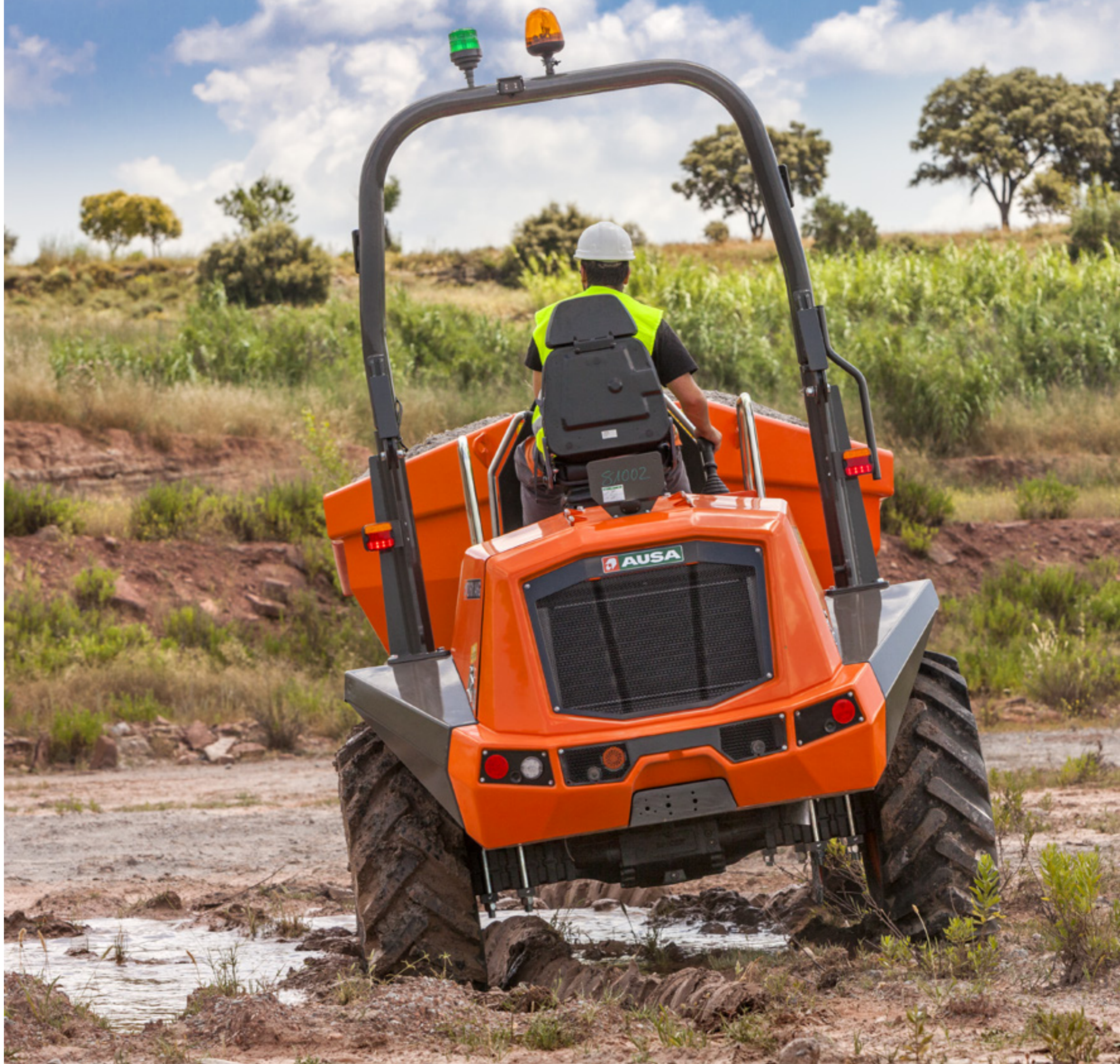
D1001APG 10000KG UNLOADING SYSTEM ROTATING POWER 55.4KW WIDTH 2,410MM TRANSMISSION TORQUE CONVERTER
