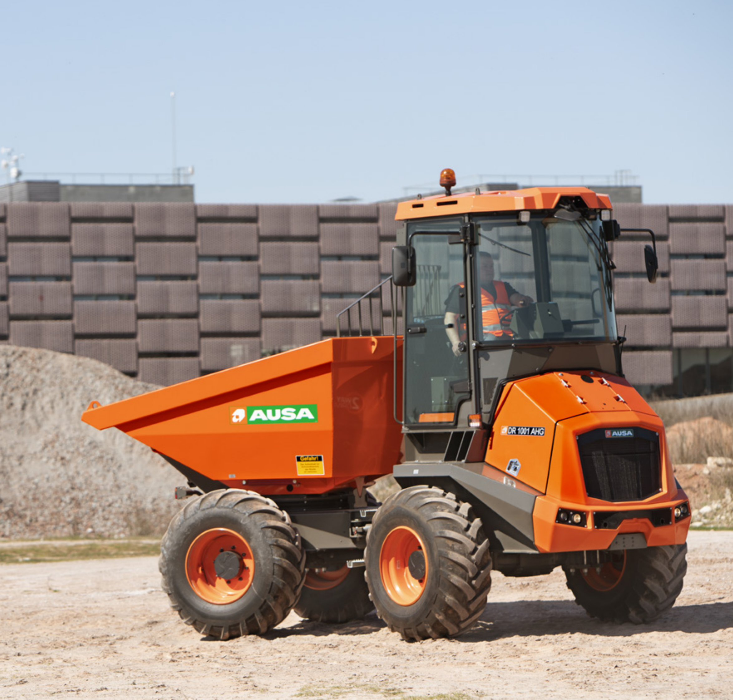
DR601AHG 6000KG UNLOADING SYSTEM ROTATING POWER 55,4KW WIDTH 2,210MM TRANSMISSION HYDROSTATIC
