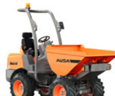
D120AHA 1200KG UNLOADING SYSTEM HIGH POWER 15.6KW WIDTH 1,210MM TRANSMISSION HYDROSTATIC
