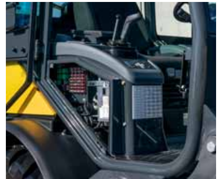
Side cover for quick maintenance access
